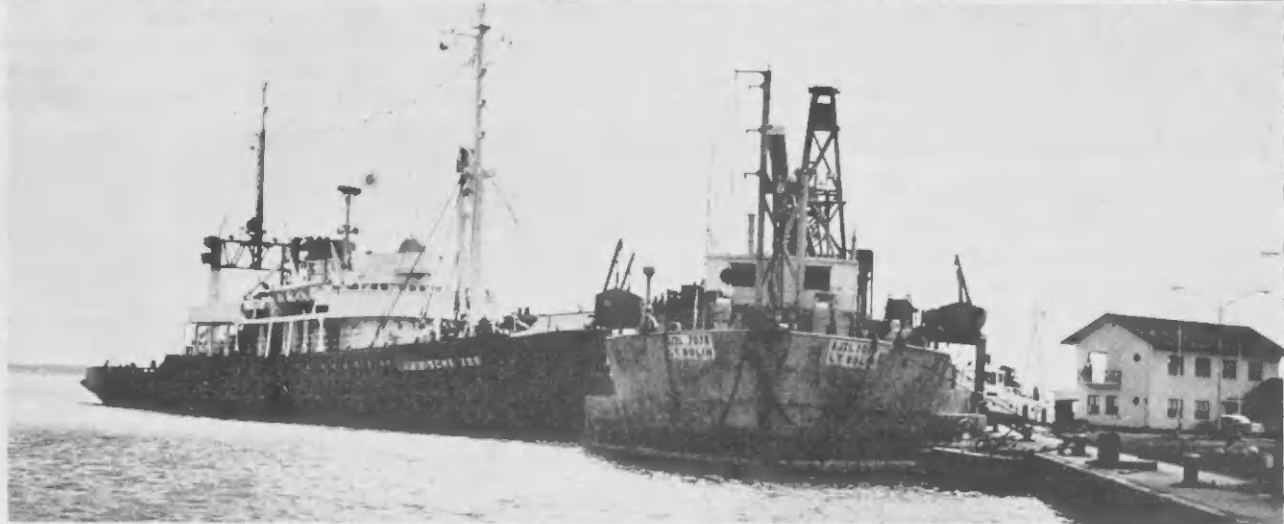
THE CARIBISCHE Zee is the largest tug in L. Smit & Company's International Tug Service. Of the twenty-two ocean-going tugs in the fleet, the Caribische Zee is the biggest and most powerful. Rated at 4500 horsepower, the vessel has a crew of twenty-six of which seventeen are Netherlands Antilleans. Stationed at Curaçao, it stopped at Aruba recently to pick up a drilling barge for a tow to Houston, Texas. Captain of the vessel, upper right, is P. W. J. de Koe.
